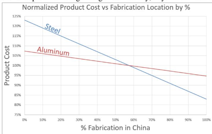
**FIGURE 3.** Cost Reduction Percentages for Steel and Aluminum with a Chinese Supply Chain
