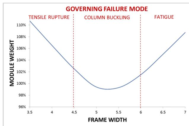
**FIGURE 4.** Frame Width vs Module Weight, Presenting Governing Failure Mode
