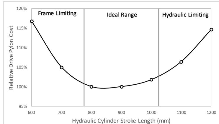
FIGURE 8. Optimization of Hydraulic Drive System
