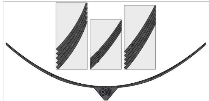
**FIGURE 7.** Parabolic Rib Nesting Profile and Final Assembly
