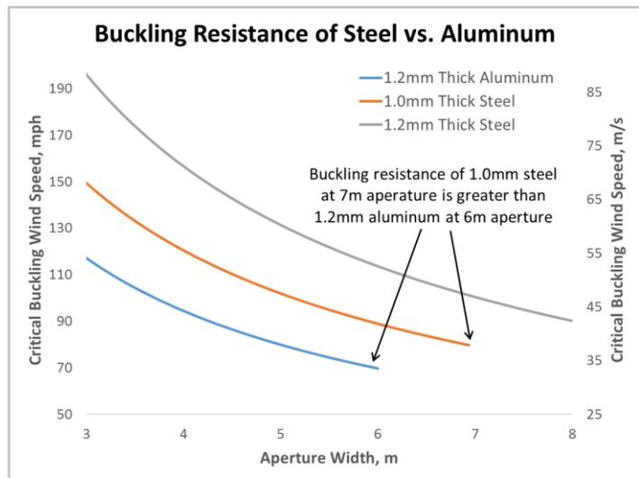
FIGURE 5. Buckling Resistance of Steel and Aluminum Reflector Sheets as a Function of Aperture and Wind Speed
