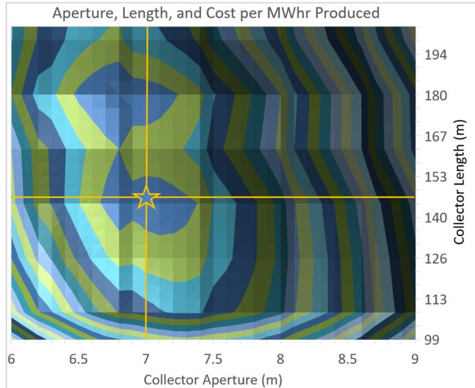
**FIGURE 2.** Result of System Design Analysis, Yielding an Optimum Collector Size of 7m Aperture x 146m Length
