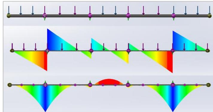
**FIGURE 6.** Parabolic Rib Loading Condition and Resulting Shear and Moment Diagrams
