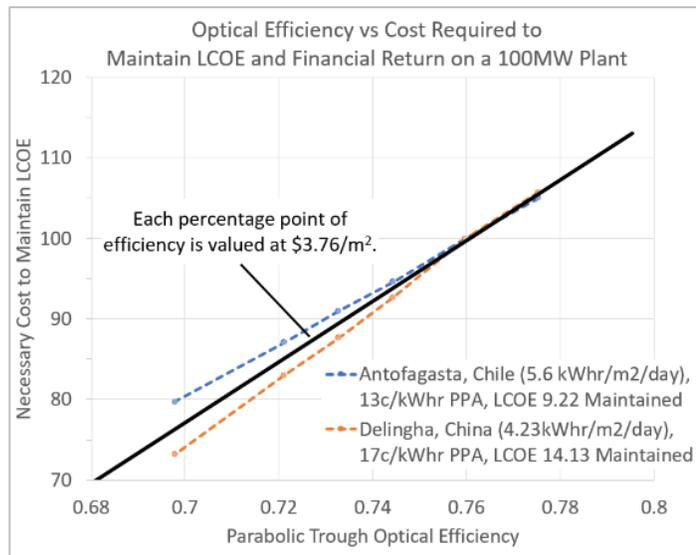
FIGURE 1. Optical Efficiency Required to Maintain LCOE and Financial Return on a 100MW Plant
