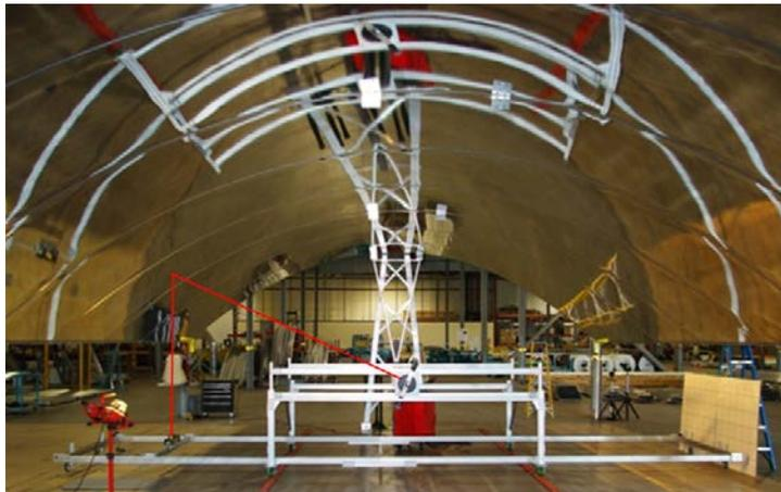
Fig. 2: Inverted SkyTrough<sup>®</sup> DSP module with test sled in position beneath the optical surface.
