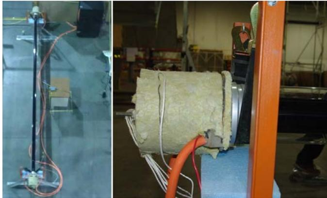
Fig. 4: Thermal receiver efficiency test stand.
