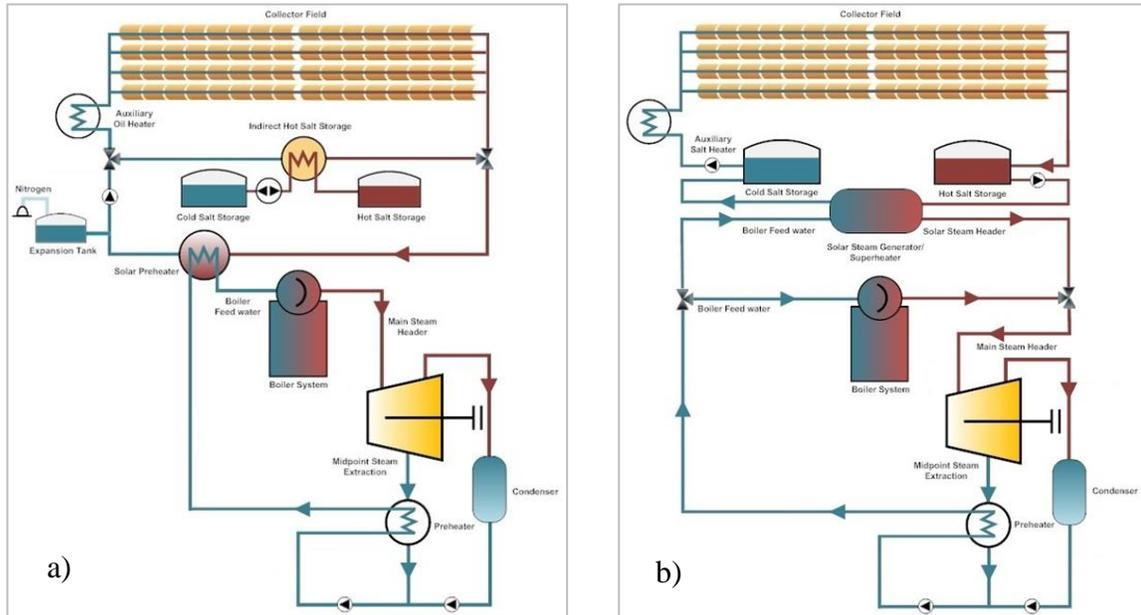
**FIGURE 2:** a) Low-Temperature (Oil-Based) Hybridization Schematic, Yielding 3% Total CSP Hybrid Addition, vs. b) High-Temperature (Molten-Salt-Based) Hybridization Schematic, Yielding 20% Total CSP Hybrid Addition
