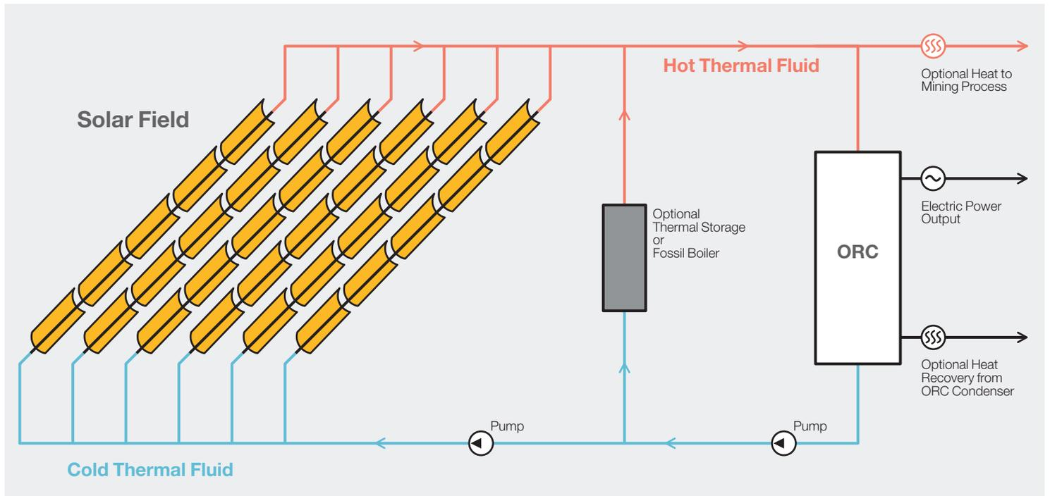
Schematic of Solar Thermal Integration with Mining Operation
