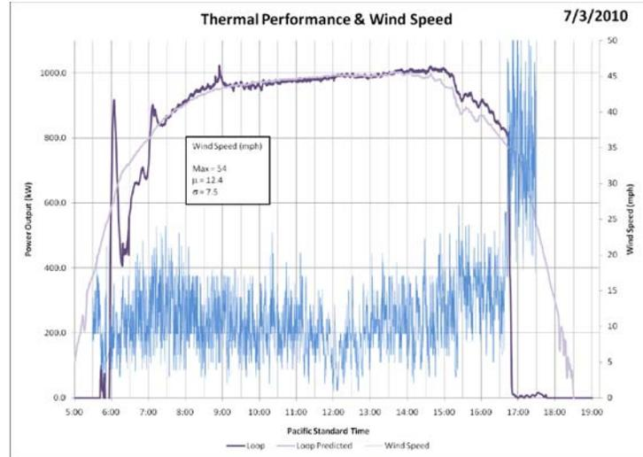
FIGURE 4. Thermal performance, predicted and measured, with wind speed for a single day.
