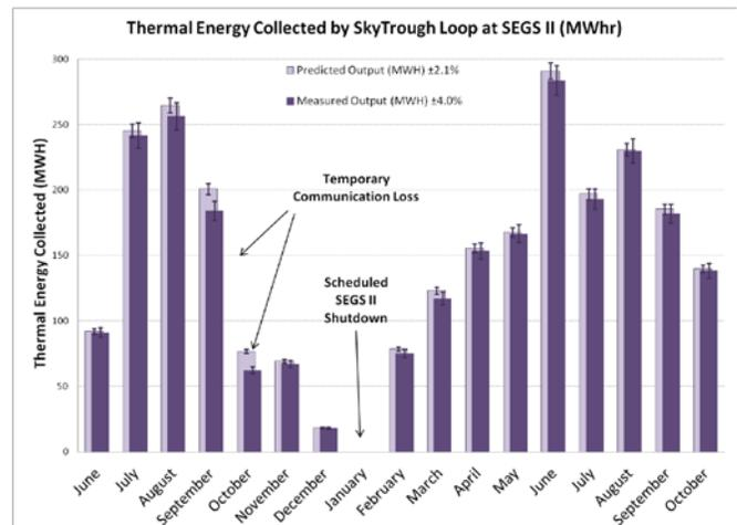
FIGURE 4. Measured compared to predicted performance of SkyTrough loop by month.
