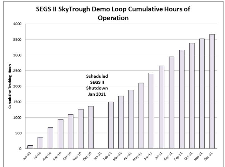
FIGURE 3. SkyTrough cumulative hours of operation, since installation of the data acquisition system.
