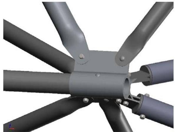
**Figure 4 – Solid model of a typical joint on the SkyTrough**
