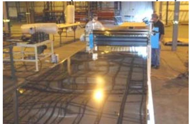
utilize a 0.05 inch thick aluminum substrate. This translates to a weight per square meter of reflective surface of 3.5 kg/m<sup>2</sup> (~0.72 lbf/ft<sup>2</sup>) versus 10 kg/m<sup>2</sup> (2.1 lbf/ft<sup>2</sup>) for glass mirrors. The use of ReflecTech® Mirror Film laminated (see Figure 7) onto an aluminum substrate allows for a lower cost, lightweight durable mirror when compared to traditional glass mirrors.
