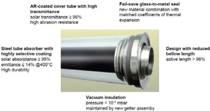
Figure 8 – Typical section of a Schott solar receiver
