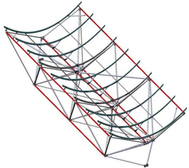
**Figure 3 – Solid model of the frame with the mirror mounting ribs shown.**
