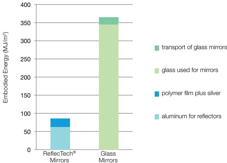
**ReflecTech®-mirrors** have a cradle-to-grave embodied energy that is **four times lower** than curved glass mirrors.
